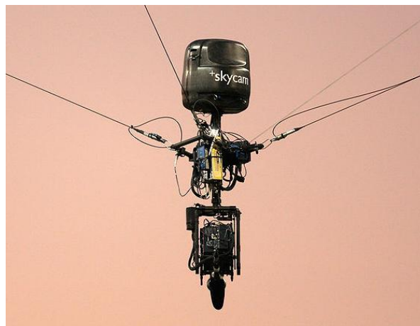
Figure 6 Skycam: a commercialized suspended cable robot
